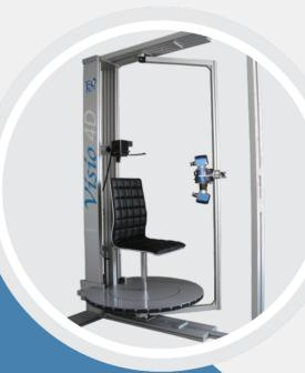
Body measurement requires 360° view of the volunteer body part. 4 to 9 views are necessary to access to all regions specially for the inner part of the legs. Local zones can be extracted from the body part for dimple analysis for instance. A very unique configuration system should be used to provide such measurement ( AEVA-HE-450 with Visio-4D bench).
